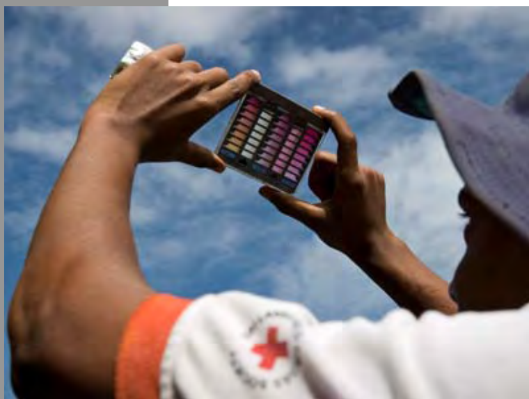
A Sri Lanka Red Crescent Society volunteer checks the chlorine content of water during the tsunami operation.- Photo: Christoffer Regild International Federation
